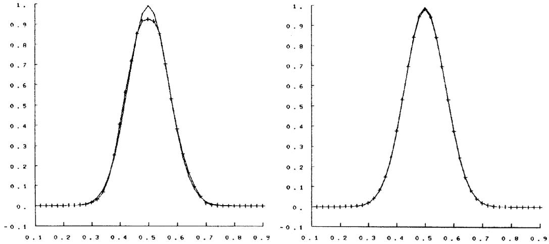
Figure 6. Numerical results with new flux limiter (left) and Holly-Preissmann (right) schemes
