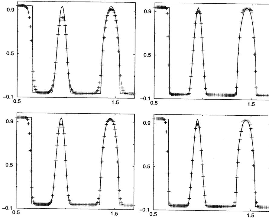
Figure 5. Comparison of results obtained on three benchmark problems at  $N_{\text{CFL}} = \frac{1}{2}$  with minmod (top left), superbee (top right), Van Leer (bottom left) and present (bottom right) limiters
