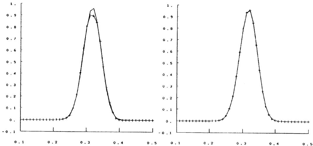
Figure 7. Numerical results with new flux limiter (left) and Holly-Preissmann (right) schemes
