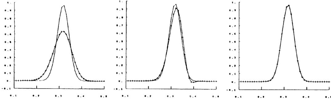
Figure 2. Comparison of first order (left), second-order (middle) and Holly-Preissmann (right) interpolations
